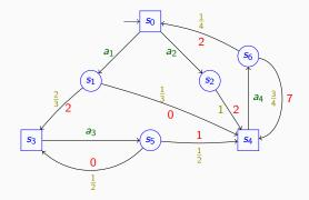
\* Play in the MDP: s<sub>0</sub> <sup>a<sub>1</sub></sup>→ s<sub>1</sub> <sup>2</sup>→ s<sub>3</sub> <sup>a<sub>3</sub></sup>→ s<sub>5</sub> <sup>1</sup>→ s<sub>4</sub>... Total cost: 3
